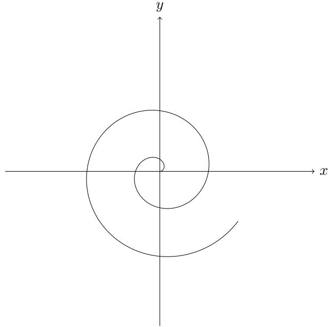
$$\begin{aligned}L(\mathbf{c}) &= \int_0^b \sqrt{a^2 + a^2\theta^2} d\theta \\&= a \int_0^b \sqrt{1 + \theta^2} d\theta \\&= \frac{a}{2} \left( b\sqrt{b^2 + 1} + \sinh^{-1} b \right)\end{aligned}$$
