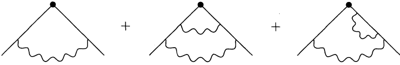
Figure 18.1. Diagrams giving the leading logarithmic contributions to the momentum dependence of the quark effective mass.
